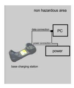
The Bluetooth handheld scanner can also be used separately in the hazardous area. The base or charging station is then operated in the non-hazardous area.
